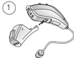
2. Once in place, move the boot in the direction of the battery compartment.
